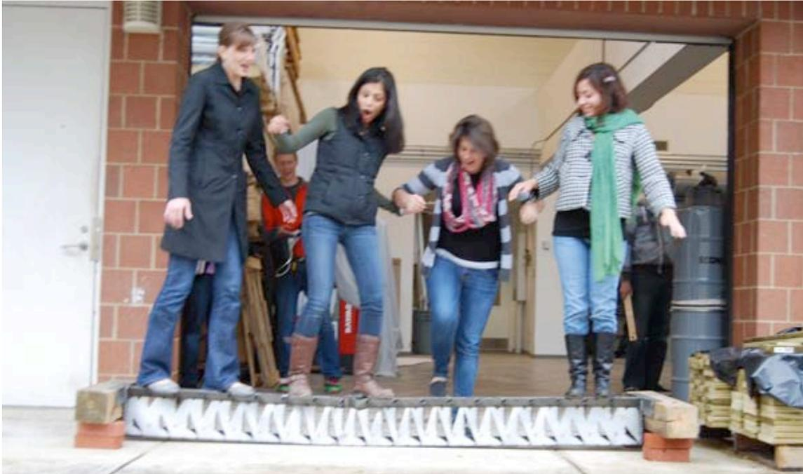
**Figure 20. After 410 pounds, the truss failed with the lower chord in tension and the upper chord in compression. (let's not acknowledge that we didn't use dead loads to do this (delete this image))**
