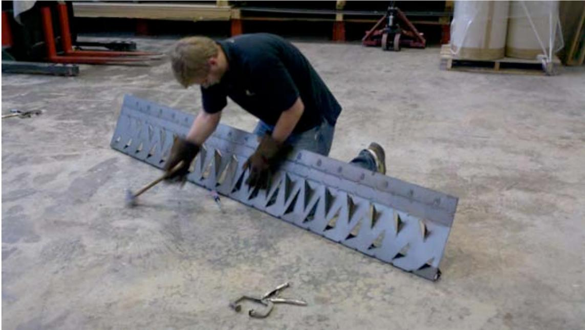
**Figure 16. The fabrication of test beam was difficult because of the heavy gauge and stitching pattern. Note the hammer.**
