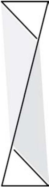
**Figure 9. Side elevation of folded base truss. Triangular fins (webbing waste) fold out to support the chords.**
