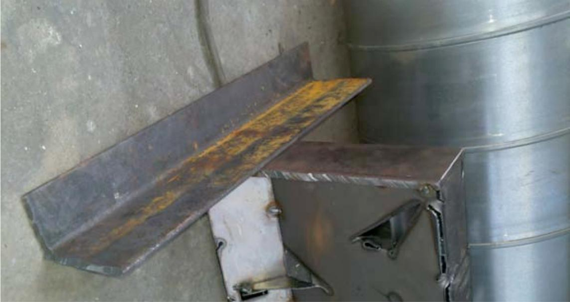
**Figure 19.** A 1/8” steel plate was welded to the end of the truss, along with a steel angle for loading and testing.
