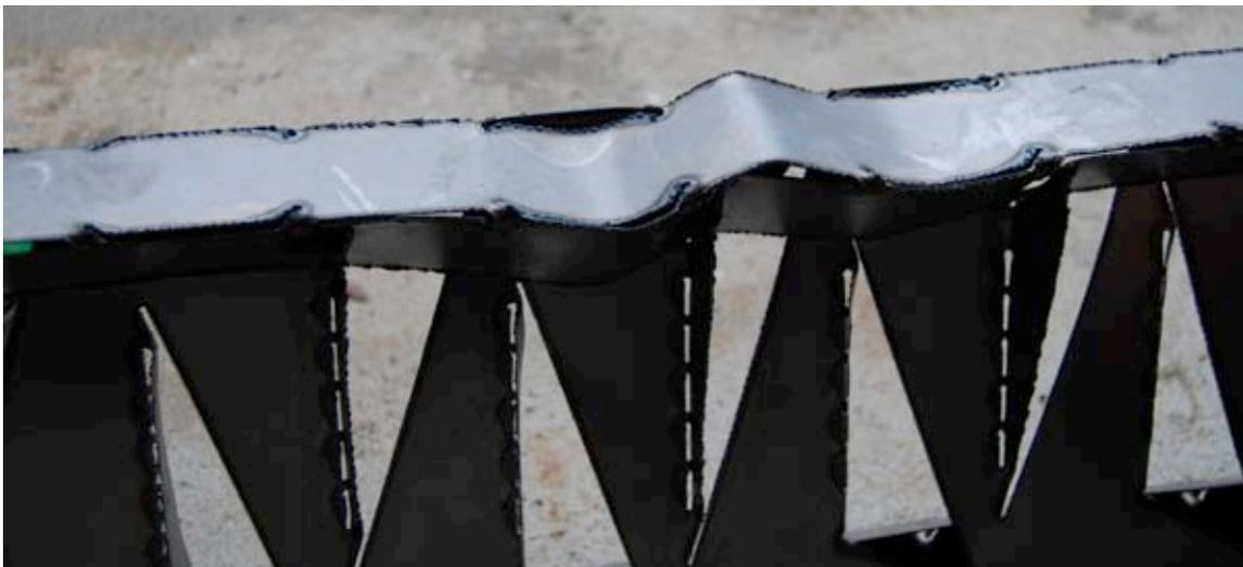
**Figure 21. The deformation of the top chord of the truss.**
